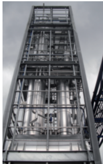
Skid-mounted unit with a falling film evaporator as column reboiler
