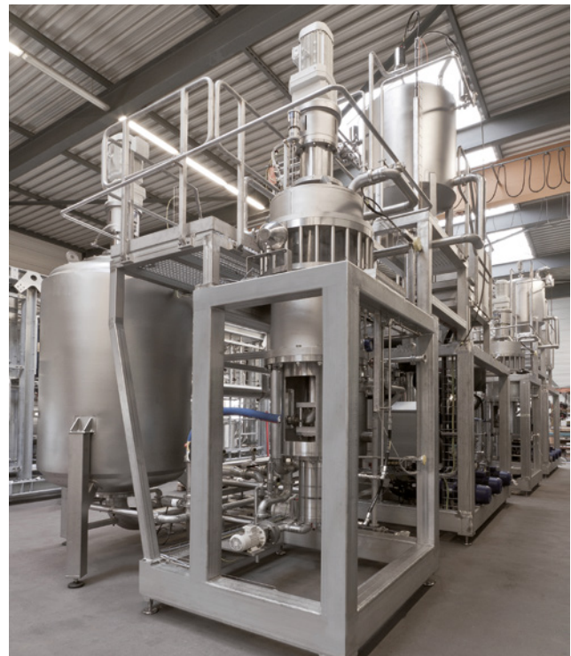
Commercial freeze concentration plant
