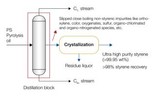
This has impact also on any future plans for scale up of recycled PS production by a client. In case of SuRe<sup>TM</sup> styrene process, due to usage of crystallization at back end, there is no requirement of blending since all these impurities are removed with ease.
