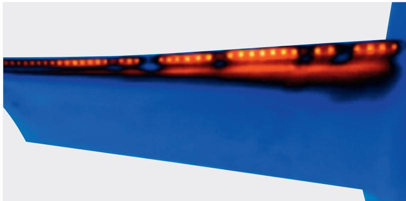
5 The thermographic measurement of a blade shows open and blocked cooling channels.
