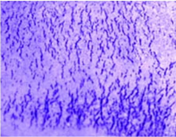
**1** Craze cracking, a typical form of damage occurring in IGT vanes (enlarged 40×).
