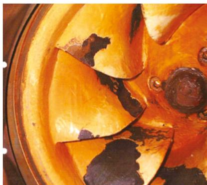
The original cavitation damaged impeller
