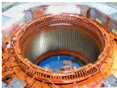
f) Stator winding completed
