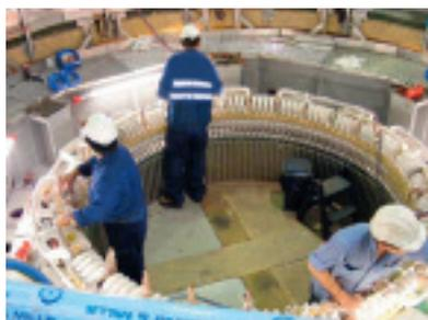
e) Stator winding connected
