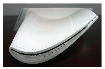
W501F R1 Blade, Fully Reconditioned and Coated with Advanced TBC
