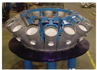
W501F Transition Repair in Full 360° Simulator Fixture
