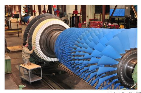
This 200 MW class gas turbine fleet has logged more than 3 million hours of operational time with many of the units now into their second major inspection cycles. To meet the demands of this maturing fleet, Sulzer Turbo Services has invested significant resources in capital, tooling and repair procedures with extraordinary standards.
