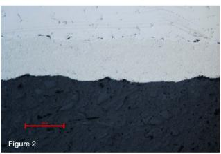
MCrAIY coatings may be utilized on both stationary and rotating components in the hot section of gas turbine engines. Examples of parts which benefit from MCrAIY coatings include turbine blades, vane segments, and shroud blocks. MCrAIY coatings can also be used as protective bond coats for yttria stabilized zirconia thermal barrier coatings. Coating thickness typically measures 5-10 mils, but can be applied in excess of 25 mils.
