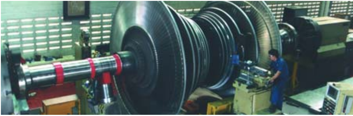
1 Besides extensive planning and skilled people, large machine tools like this 63-ton lathe are necessary for performing high-quality repairs on big rotors.
