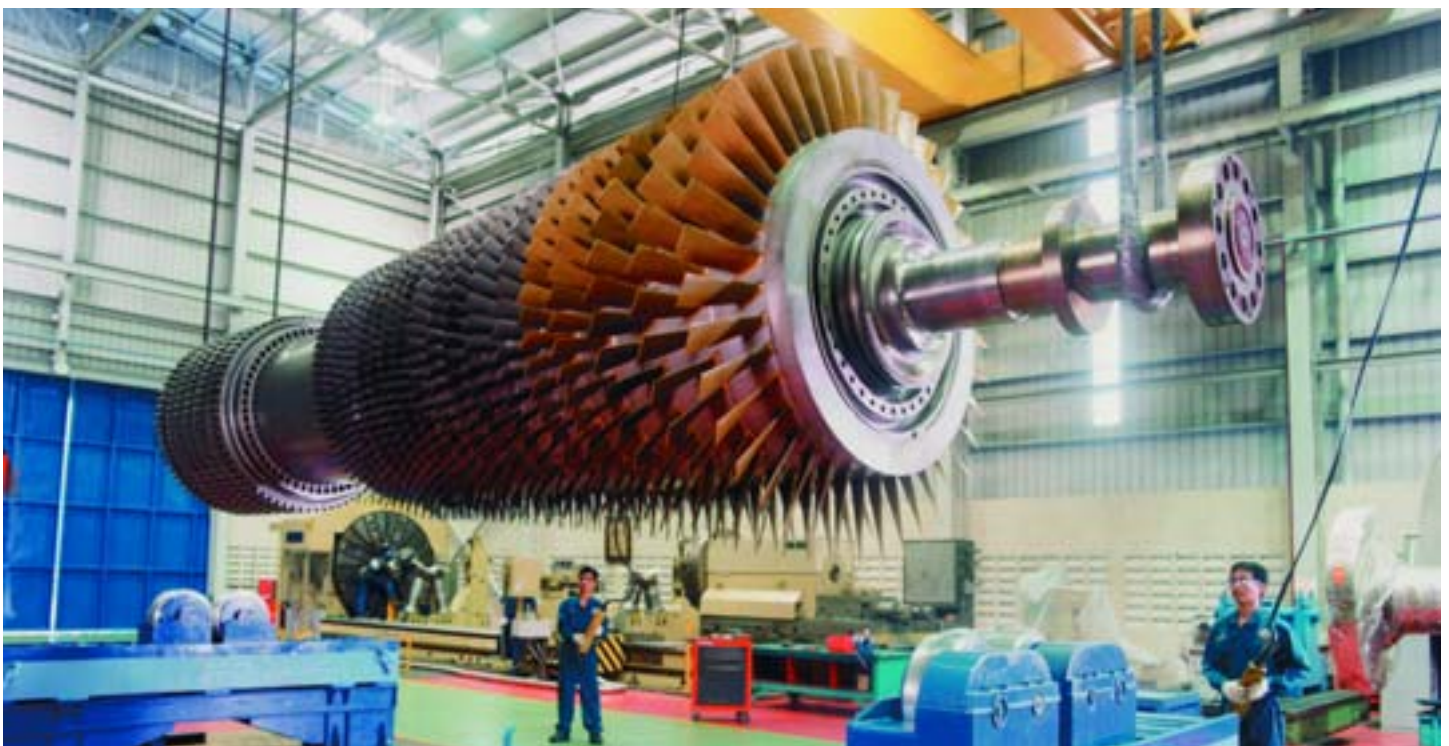
1 Rotor of a huge gas turbine which could be repaired by Sulzer Turbomachinery Services after a severe outage. The gas turbine is used in a combined-cycle power plant. The repair was faster and cheaper than a replacement.
