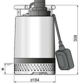
\* Continuous running water level 76 mm
