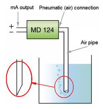
You have to consider that the majority of the mistakes using a pneumatic sensor usually happen due to pipe clogging or due to air losses in the pipe or/and pipe junctions; if you are going to use a prefabricated sump made by ABS without this inlet and with an APC control panel with MD 124 pneumatic sensor, make sure to avoid pipe clogging as making a diagonal cut to the air pipe to have a bigger area of the side of the pipe submersed (as it is shown at the left side picture).
