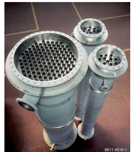
Falling film evaporator tubes
