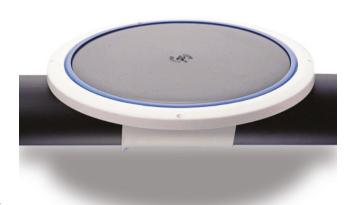
When the air flow is turned off, the pressure of the water above presses the membrane disc tightly to the main body closing the small slits on the membrane. The non-return valve with a stainless steel ball pushed down firmly to an o-ring seal inside makes sure that no water enters the pipeline. During normal operation the non-return valve also works as a control orifice.
