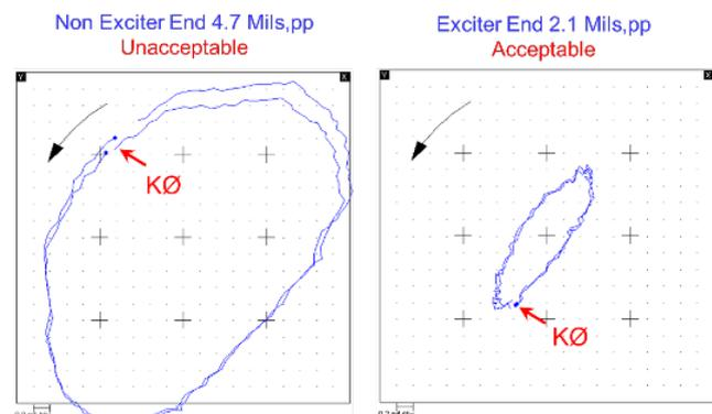
Based on the physical characteristics of the generator, a conservative 16 ounce calibration weight was installed at the non exciter end. The unit showed good improvement and balance sensitivity vectors were computed. Based on these vectors, a final correction weight was computed, and a 23 ounce weight was installed 60 degrees from the initial calibration weight. The positive results of this final weight addition are displayed in the adjacent orbit plots.
