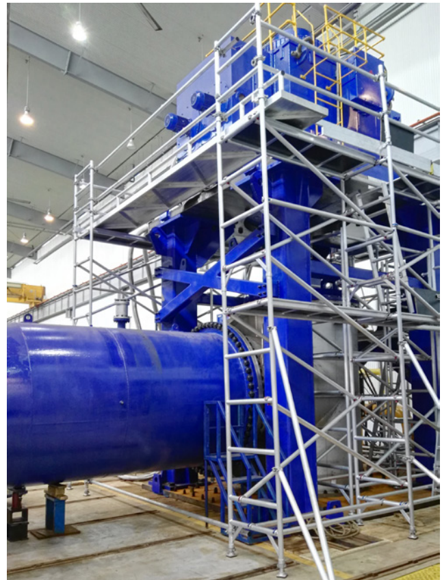
Large vertical circulating water pump on Sulzer's test bed
