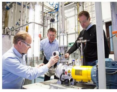
Hydraulics, impeller, seal, pump design and material - many factors together influence the operation of the pump, in addition to the fluid being pumped and the process temperature. These features can be tested in the demo loop, here presented by (from the left) Jukka Vanhala, Matti Rikka and Saku Vanhala.
