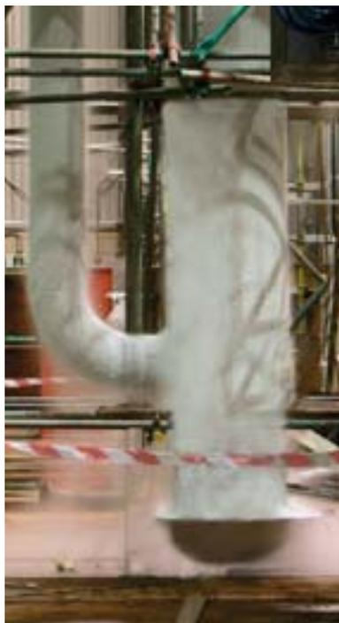
**4** Liquid nitrogen cold spin test.
