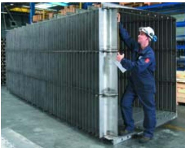
Separators made of wire mesh (mesh-demisters) form the subsequent agglomeration stage. These are operated at high gas load factors, which bring about flooding of the mesh packing (Fig. 2). During this coalescence stage, agglomeration of very fine drops results in larger drops that can then be separated without problem in the next Swirldeck stage (Fig. 3). The separated liquid is collected and led into the column sump through drain pipes.
