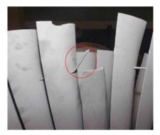
Blade failure caused by vibratory fatigue
