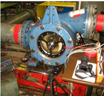
Test on a scale down model of a boiler feed water pump with diffuser
