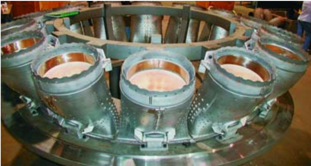
**1** These fixtures simulate the transition piece fit-up in the turbine, thus ensuring repeatability and accuracy of transition piece repairs.
