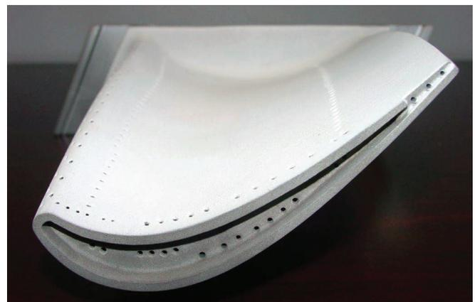
W501F R1 Blade, Fully Reconditioned and Coated with Advanced TBC
