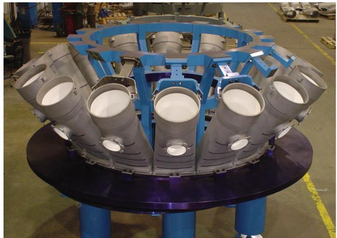
W501F Transition Repair in Full 360° Simulator Fixture
