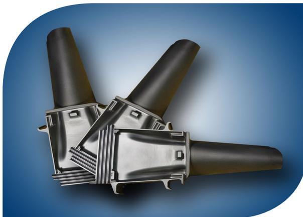
The thickness of a typical MCrAlY coating (.006-.010 inches) is up to four times greater than that of an Al or PtAl coating. Due to increased coating thicknesses, there are larger amounts of critical elements (aluminum and chrome) available to form protective oxide layers. Also, unlike diffusion coatings, MCrAlY's are not dependent on substrate chemistry.
