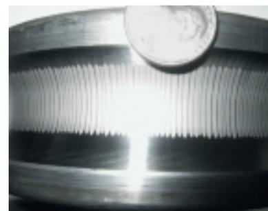
5 Photo of the bearing damage detected by the vibration data in figure 4.
