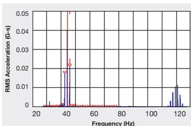
provides a database, which, by reviewing vibration trends, is helpful in predicting mechanical problems in rotating machines and estimating future maintenance needs, extending the duration between inspections, and minimizing downtime for maintenance.
