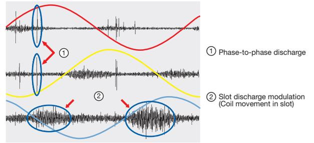
7 The discharge levels on one of the machines suggested phase-to-phase discharge (RED and YELLOW phases). There was also evidence of slot discharge modulation—most pronounced in the blue phase.
