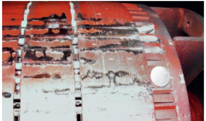
Photo of the damaged rotor “called” from the vibration data in figures 1 and 2.
