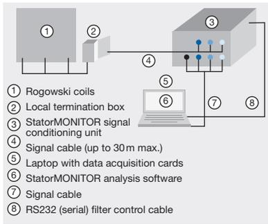
6 Typical test setup for partial discharge using the StatorMONITOR system.
