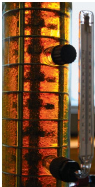
[3] Agitated liquid-liquid extraction column in pilot scale.
