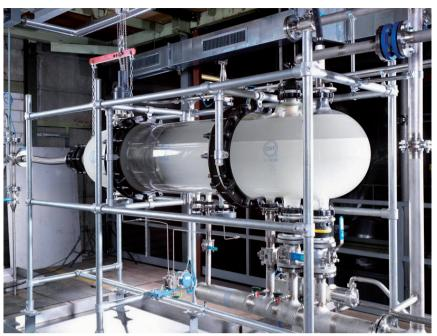
Fig. 18a: Test rig for Sulzer Mellaplate and DC Coalescer
