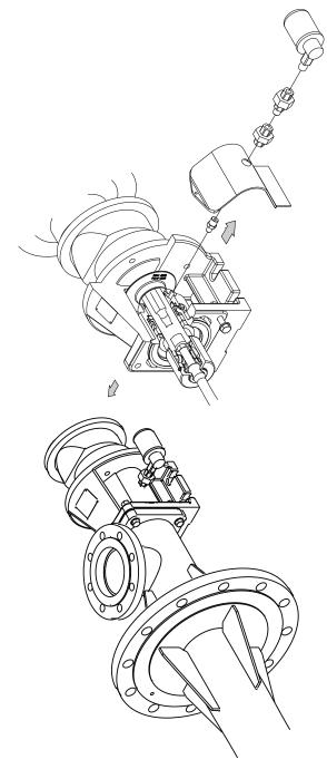
Figure 1. Fitting of constant level oilers.
