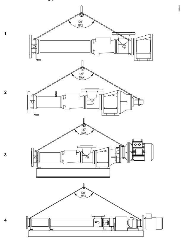
Figure 2. recommended lifting points
