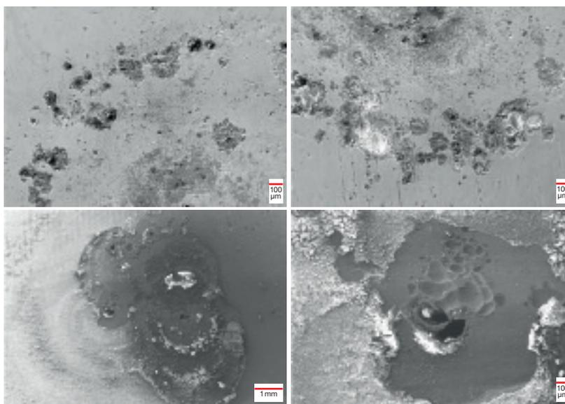
② Piping made from high-alloy stainless steel with clearly visible pitting corrosion.
