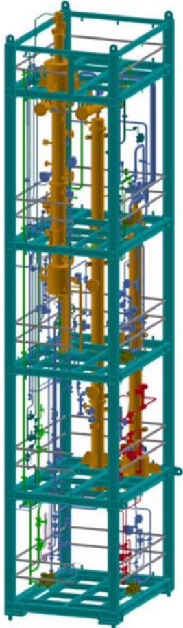
Scrubber for Amine or Glycol Treatment
