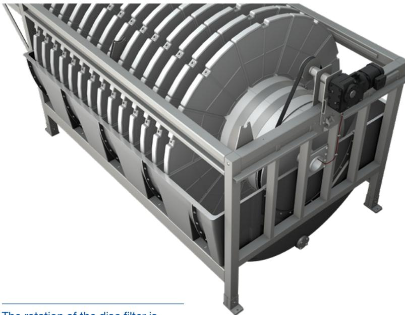
When the water level inside the filter discs increases to a preset point, the filter rotor starts rotating and the backwash of the filter cloth starts. The high pressure backwash spray nozzles remove the accumulated suspended solids into the reject trough inside the filter. The suspended solids are discharged by gravity.
