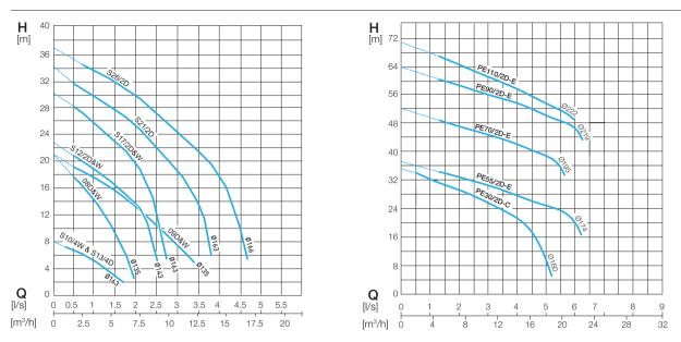
H = Total Head Q = Discharge Volume. Curves to ISO 9906 (60 Hz available on request). N.B. please use the ABSEL program to validate pump selection.
