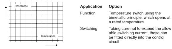
Curve showing principle of operation of bimetallic temperature limiter
