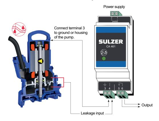
Sulzer leakage control type CA 461
