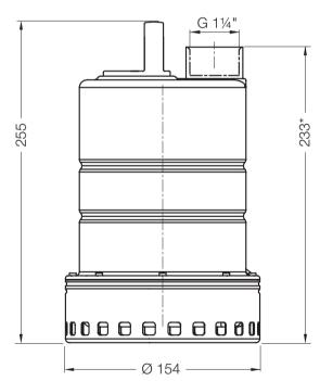
\* With discharge adaptor kit: 310 mm (when replacing Coronada 200)
