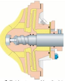
3 The inherent pressure of the medium being handled ensures the seal in the standstill condition. The internal pressure in the pump, however, must be higher than the atmospheric pressure.
