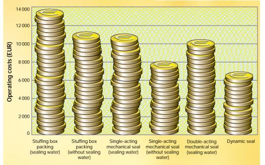
Within a period of ten years, a conventional stuffing box packing results in costs amounting to almost 14 000 Euro. The cost of operating a dynamic seal is only 50% of this figure (Assumptions: 0.08 EUR per m³ sealing fluid, 0.045 EUR per kWh energy).
