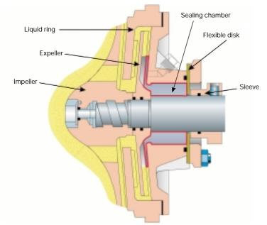
2 During the operation of the pump, an auxiliary wheel pumps the medium being handled out of the sealing chamber. The operating costs of a dynamic seal are lower than those of a conventional seal.
