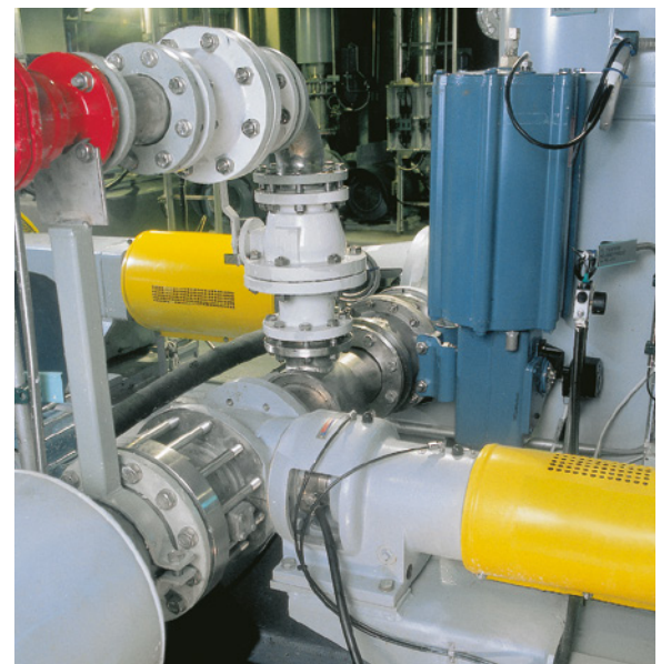
Fig. 28. ClO 2 mixing with chemical mixer.
