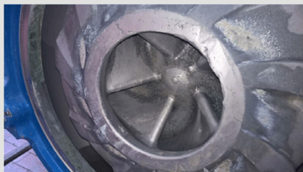
Figure 6. Close inspection shows no significant wear during the test period
