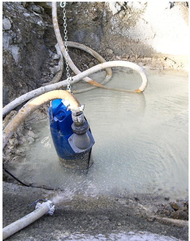
The Sulzer submersible drainage pumps XJ are ideal for pumping water and dirty water mixed with soil. When delivered to a site you can start using them right away. Pumps with a built-in AquaTronic unit will always have the correct direction of impeller rotation, ensuring peak performance and reduced wear.
