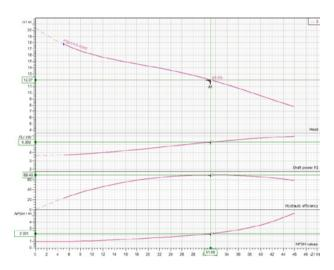
The XFP100E has a class-leading solids throughlet of 80 mm, whilst maintaining a hydraulic efficiency of ~70%. The PE60/4 IE3 Premium Efficiency motor completes the package at 91%.
