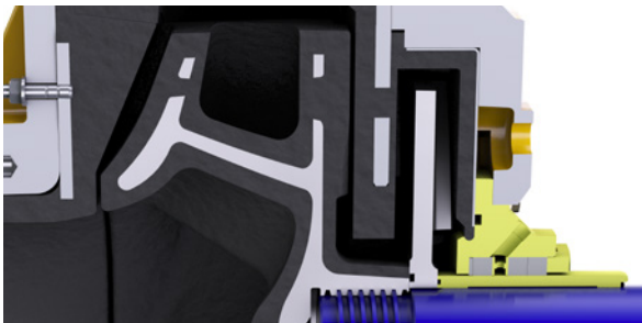
Separate and removable suction plate (from size 200).
