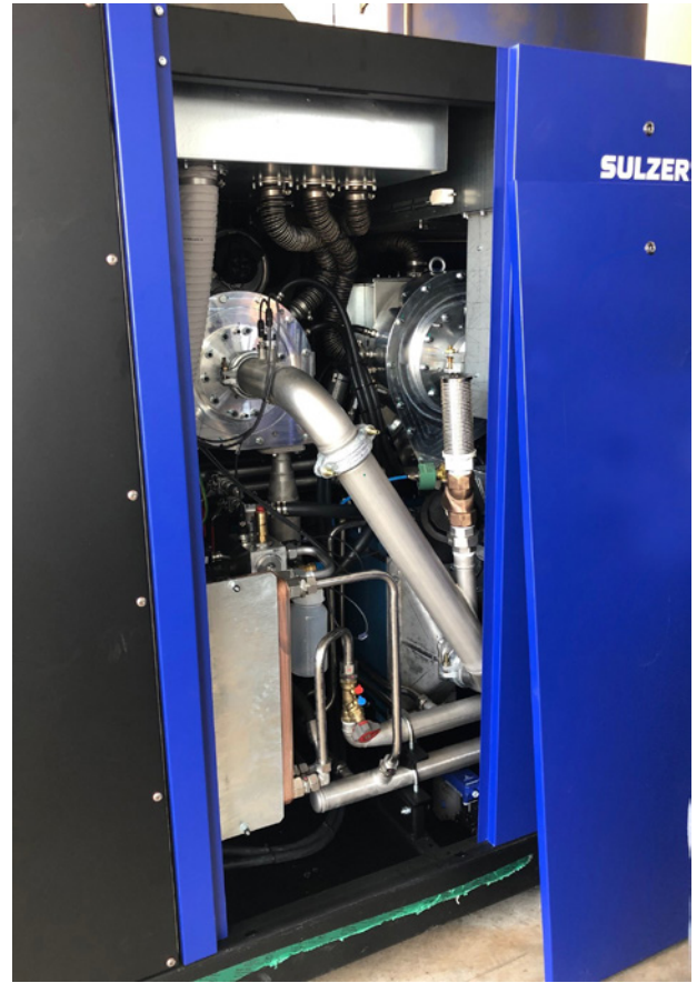
This is how it looks inside a HSR turbocompressor.
