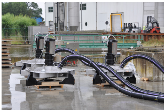
OKI aerator mixers are fast and easy to install.
