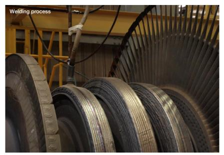
Welding preparations were performed prior to the welding process. A detailed Stress analysis was performed to determine the stress distributions especially in the disk area. By knowing the stress distribution, the Heat Affected Zone (HAZ) can be positioned in the low stress area. Stage 2, 3 and 4 disk steeples were then machined out. After successful Non Destructive Testing (NDT), the rotor was ready for the welding process.
