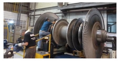
All blades were moment weight prior to installation. The moment weighing will determine the blade distribution in order to minimize residual unbalance at each stage. The blades were then installed in the rotor disks and locked in place. Progressive balancing was performed during the installation process.
