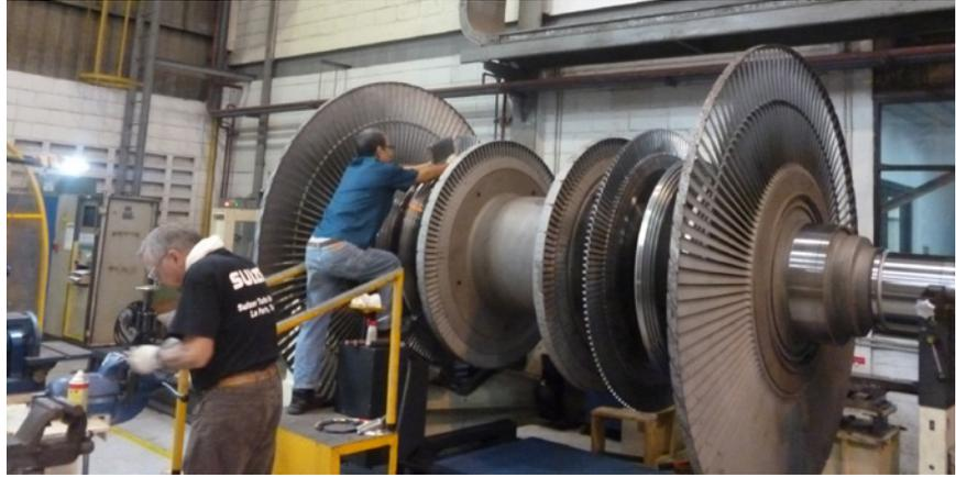
All blades were moment weight prior to installation. The moment weighing will determine the blade distribution in order to minimize residual unbalance at each stage. The blades were then installed in the rotor disks and locked in place. Progressive balancing was performed during the installation process.
