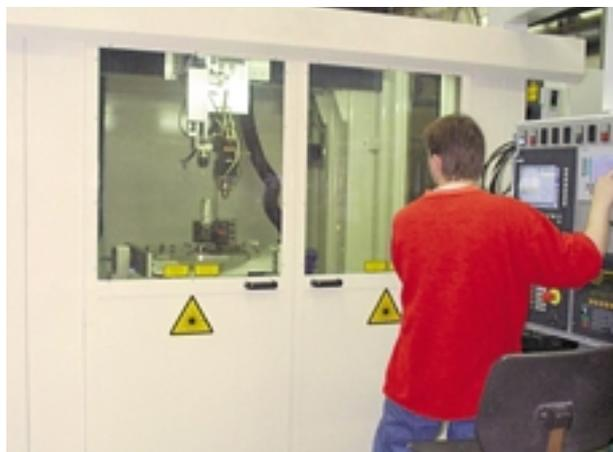
2<sup>■</sup> The Sulzer Elbar laser center combines a welding and cladding technique for the repair of gas turbine components.
