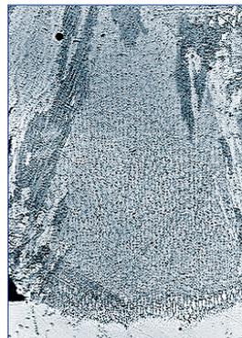
6<sup>■</sup> The microstructures change from the center to the flanges, depending on the cooling rate.
