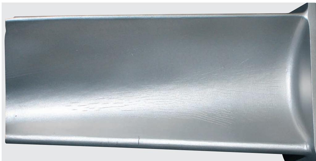
2 First-stage blade after coating removal and cleaning. It exhibits thermal cycling cracking in the leading edge and on the airfoil.
