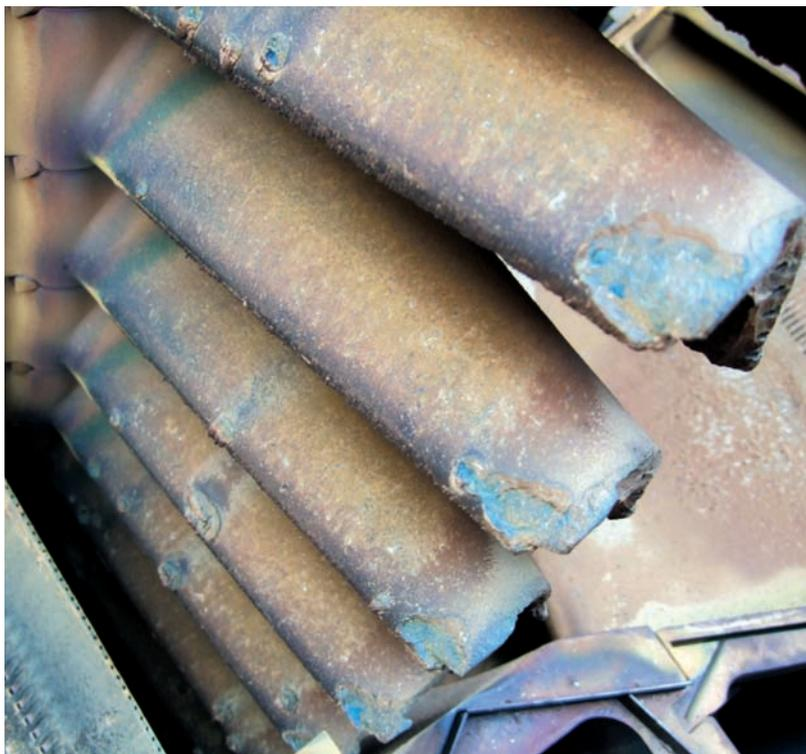
4 Hot Corrosion damage in first stage gas turbine blades.
