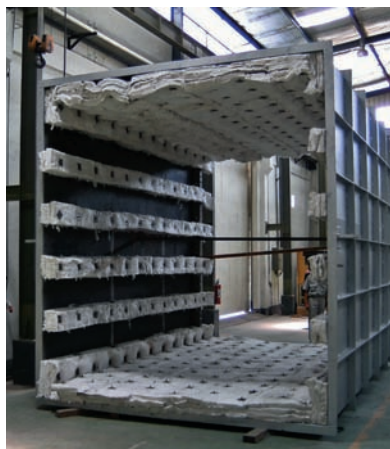
⑦ The exhaust silencer modules were fabricated according to specifications from Sulzer Turbo Services.
