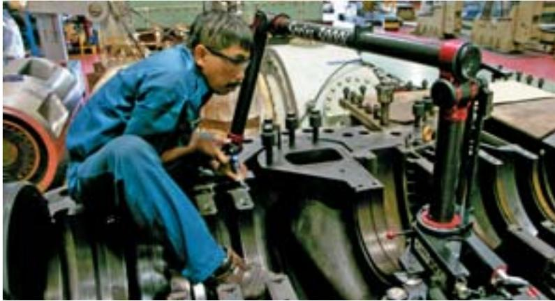
**3** The blade parameters required for the meanline modeling, including the hub and casing radius and axial locations of the leading and trailing edges of all blade rows, were acquired using a portable coordinate measuring machine (CMM).
