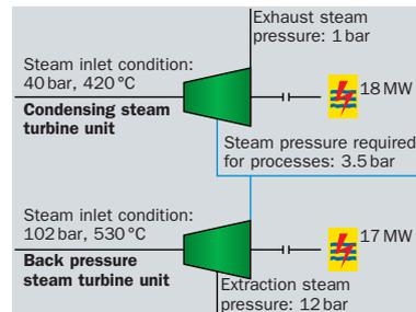
**2** Process steam of 3.5 bar is taken from the 2 steam turbine units as extraction steam (unit 1) and exhaust steam (unit 2). Sulzer Turbo Services carried out a study to demonstrate that they can operate safely at this condition.
