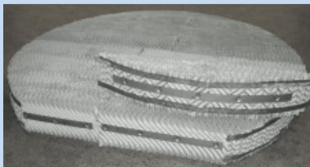
1 Sulzer AYPlus™ DC packing: ready for installation in an industrial distillation unit.
